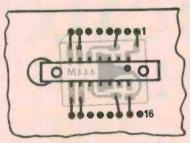
Fig. 2. Component overlay showing how the small board is connected.
