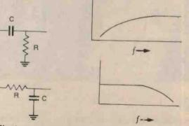
Fig. 2. Simple low-pass and high-pass filters. The signal will be 3 dB down at the frequency where  $X_C = R$ .
