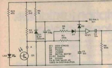
Fig. 5. Changes needed to the circuit to use light beam points.
