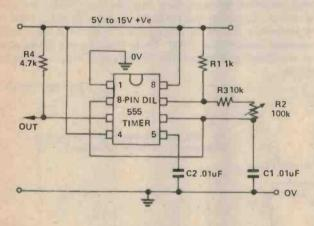
Fig. 15: Variable frequency square wave generator covers the range 650Hz - 7.2 kHz approximately.
