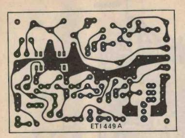
Fig. 3. Printed circuit layout. Full size 90 x 65 mm.
