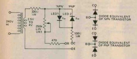
A diode can be checked by connecting it between C and E. If LED 1 lights the diode is OK and its anode is connected to C. If LED 2 lights its cathode is connected to C. If both light it is a short circuit suitable only as a link!
