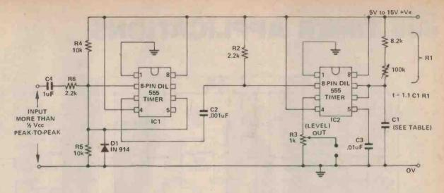
Fig. 10b: Improved add-on pulse generator is triggered by any input waveform.
