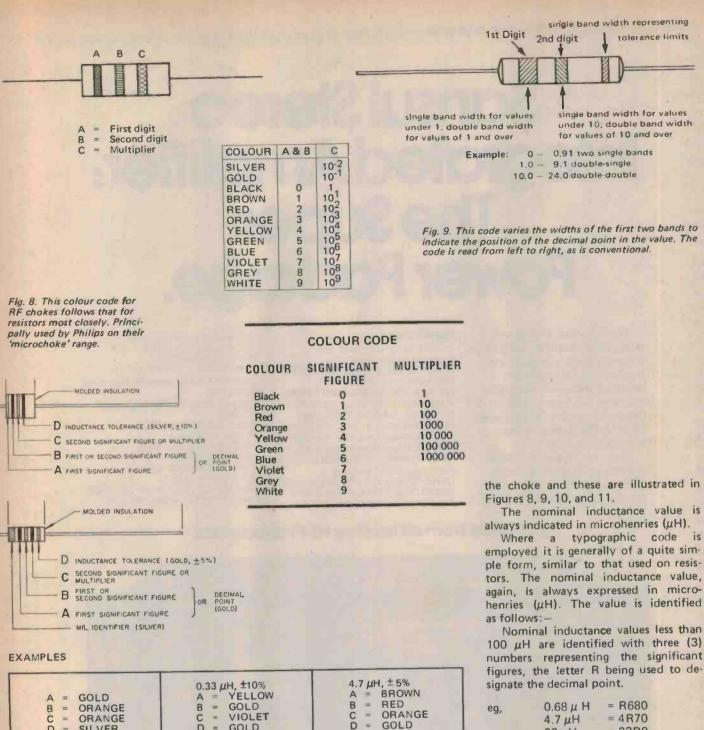
D GOLD D SILVER 15 mH, ± 5% Fig. 10. This is similar to the code in figure 8 but the decimal point for values under  $10\mu$ H is indicated by a gold band for bands A or B. A mil-Spec component is identified by broad silver band preceeding the value and tolerance bands. Some manufacturers use a dot to Indicate the
