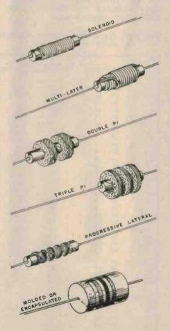
Fig. 1. General range of constructor styles of RF chokes. The particular style employed depends on the required or allowable component. Size, the inductance, the application and the required characteristics. the result that it has a very weak stray field, reducing 'crosstalk', or coupling, between the choke and adjacent components. In fact, two chokes can be mounted so that they touch each other over the full length of the bobbin – and crosstalk attenuation is quoted as 60 dB.
