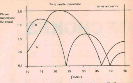
Fig. 4. Typical behavior of two RF chokes (A = around 10 µH, B = around 40 µH) over a range of frequencies.
