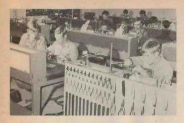
This classroom is where the trainee learns how to solder. The instructor explains a particular soldering job on the blackboard and straight away the trainee tries it out using his temperature-controlled iron.
