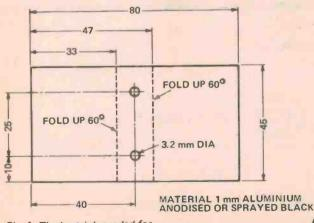
Fig. 1. The heatsink needed for the LM379S.
